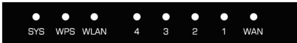
**SYS:** Flickering light indicates a proper connection to the power supply.
