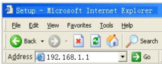
To access the configuration pages, open a web-browser such as Internet Explorer and enter the IP address of the router (**192.168.1.1**).
