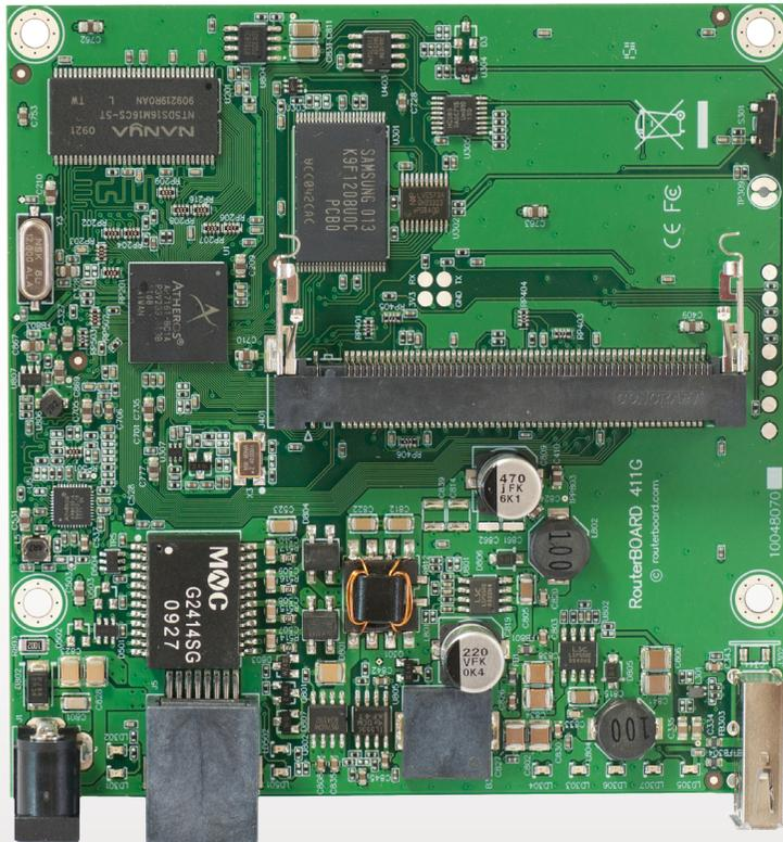
The RB400L is our new low cost series. The RB411GL has one miniPCI slot, one Gigabit Ethernet port and a USB port for 3G or storage.
